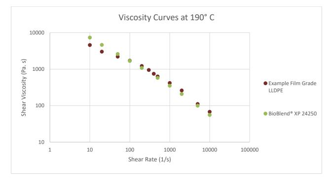
The MFI of XP 24250 is lower than the MFI of a typical blown film grade of LLDPE ( < 10 1/s). However, as shown above XP 24250 exhibits shear thinning behavior and performs closer to a standard film grade LLDPE under typical blown film conditions (200 1/s).
